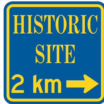
(c) G609 – Historic Site Route Marker
