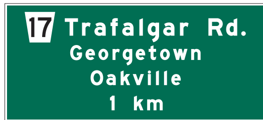
Figure 5.4: G100 – Freeway Advance Sign (Ground-Mounted)
