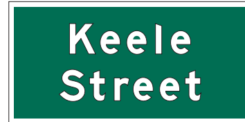
Figure 5.28: G220 – Roadway Identification (Grade Separation) Sign
