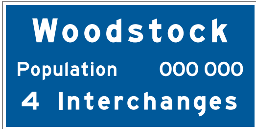
Figure 5.20: G312 – Multiple Interchange Boundary Sign (1-9 Interchanges) (Basic)
