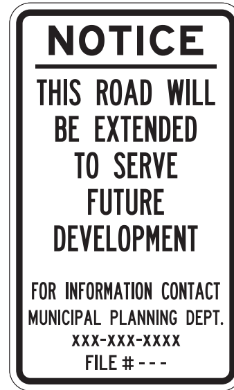
Figure 17.13: G722 – Notice – Road Extension
