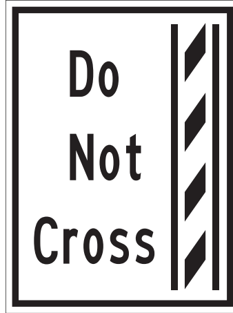
HOV – DO NOT CROSS RIGHT Sign (Ground-mounted) (HOV-4aR)
