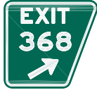
Ground Mounted Gore Sign
