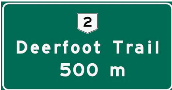
Figure 5.1 – Advance Guide Sign with Highway Route Marker
