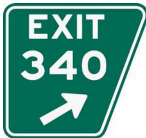
Figure 5.14 – Numbered Exit Gore Sign
