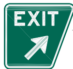
Ground Mounted Gore Sign
