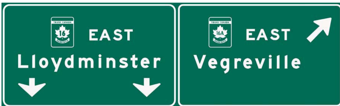
Figure 5.15 – Bypass Route (Single Exit)
