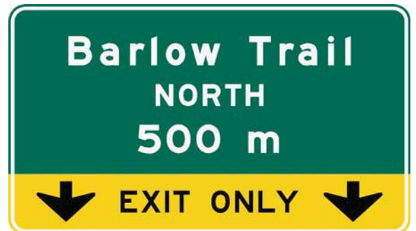
Figure 5.8 – EXIT ONLY - Double Lane Advanced Guide Sign
