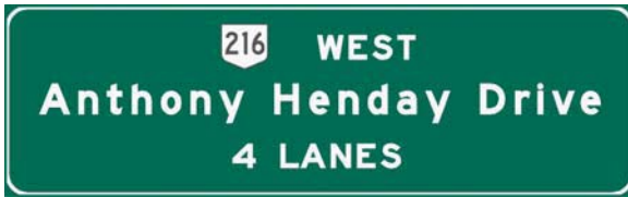
Figure 3.6 – Specific Traffic Lane (more than three lanes)
